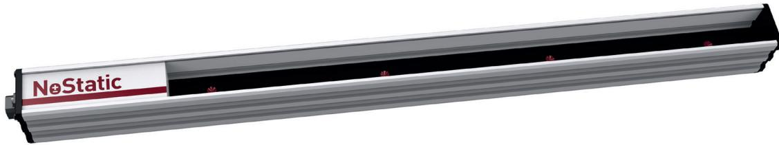
**No Static Long Range** an highly efficient antistatic system, useful in a many applications. Integrated high voltage unit, it is powered with 24VDC.
